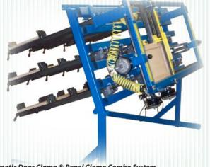
**Pneumatic Door Clamp & Panel Clamp Combo System**
