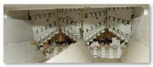
Unique infeed roller designs available, such as the above VTH 12-VU Paper Core Shredder, designed specifically for size reduction of paper cores.
