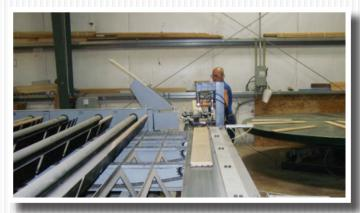
Strips of flooring are singulated and measured for length before being released into the main machine.
