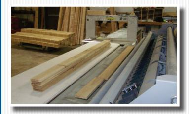
Strips are accumulated into rows. Rows are accumulated into layers. Layers are accumulated into bundles.
